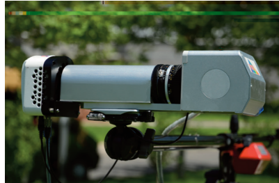
China's first field imaging spectrometer, widely applied in various fields including hyperspectral mechanism research, food security, preservation of cultural relics and target detection
