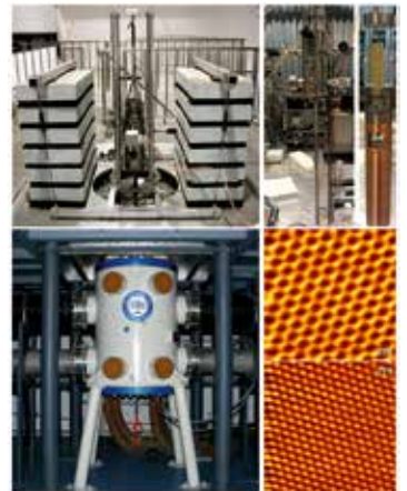
The world's only scanning tunnel microscope usable in water-cooled magnets.
