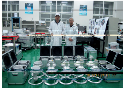
18 flight models of the HE main detectors
